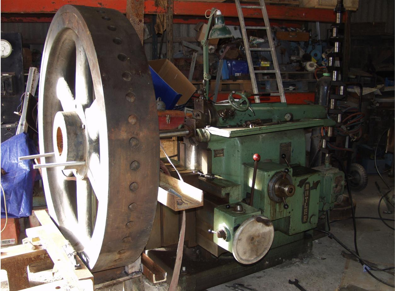
A large industrial shaper machine is shown in a workshop. A large, dark metal flywheel is mounted on the machine's table. The flywheel has a keyway being worked on by a shaper tool. The machine is green and has various adjustment knobs and handles. The workshop background is cluttered with tools and equipment. |
