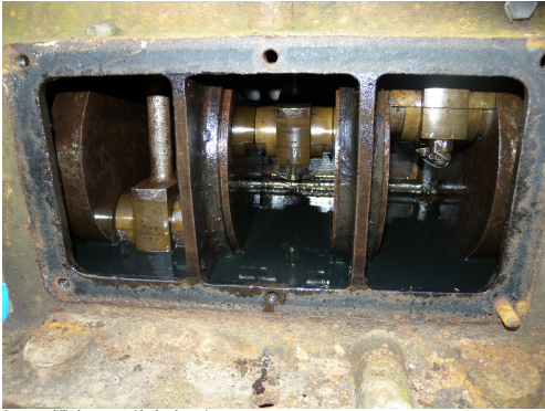
Cages were difficult to extract with a lot of corrosion
