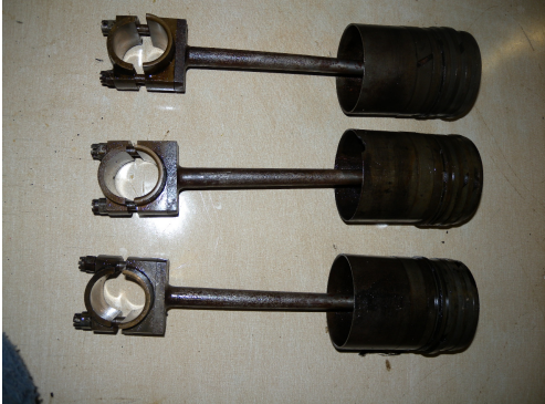
Pistons in reasonable order with little wear
