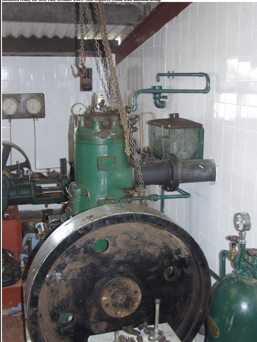
Installed ready for first run, October 2009. Still requires crank stub manufacturing.
